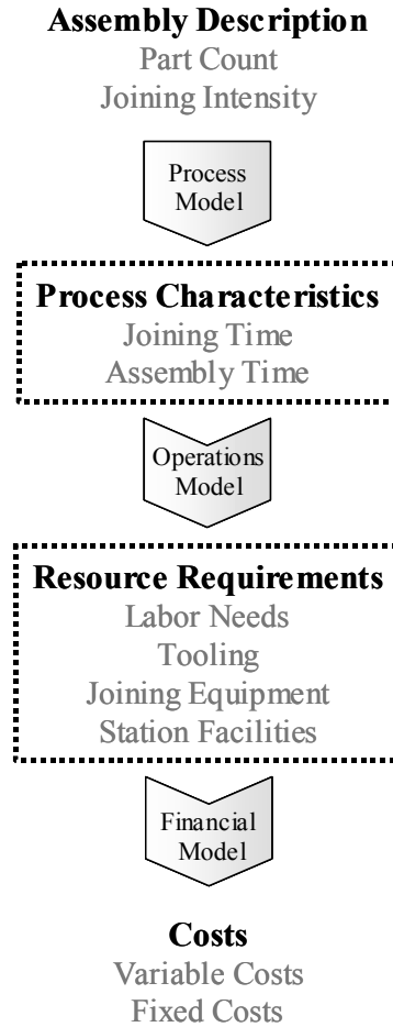
Figure 2: Schematic of Technical Cost Modeling for Assembly
