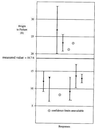
**FIGURE 15.2** Demonstration of overconfidence: The true value of the strength of the embankment, as measured by the height of the load, was outside all of the experts' 50% confidence limits.
